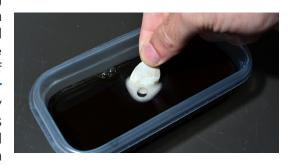
duration. If the solution has expended, the solution will not be dissolving calcium and additional **RDO Rapid Decalcifier** may be required to complete the decalcification process. However, if the solution is still active at the end of the recommended time, all of the calcium has been dissolved within the specimen and it is ready to be rinsed and fixed for observations.
